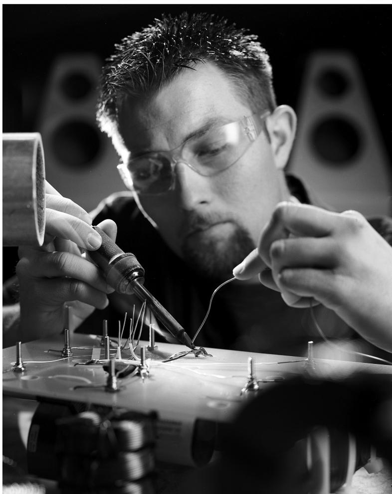
Caleb Mower is hand soldering point-to-point wiring on one of our crossovers. He's using two different types of solder: one chosen for the upper frequencies, the other for the lower. Meanwhile, most other high end manufacturers are wave-soldering their components to printed circuit boards, which are inherently poor conductors of high current music signals.
